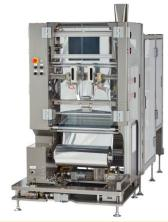
By installing a hem folding device (option), it is possible to make bag with Hem seal.
