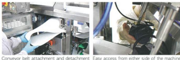
Conveyor belt attachment and detachment Easy access from either side of the machine
