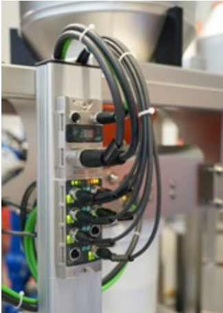
Short installation and commissioning times through simple wiring with IO-Link.
